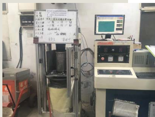
2019.04.19 The compressive strength test of concrete
