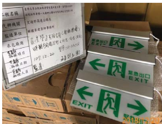
2018.12.20 The examine of fire protection indicator light
