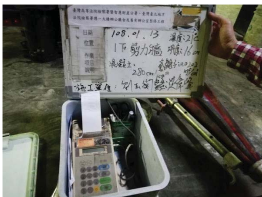
2019.01.13 The Chloride test of concrete
